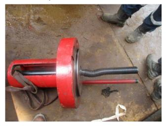
Upon further inspection of the manual locking system, it was noted that the locking shaft was damaged as can be seen in the picture on the left.
