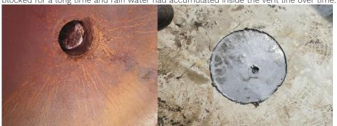
Above on the left, a picture taken from inside the mud gas separator showing the metal plate inside the vent line located at the top of the separator. On the right, the picture shows the metal plate after it had been cut and removed from the vent line.
